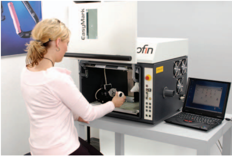
Rofin's EastMark II is one of the most compact laser marking systems on the market
